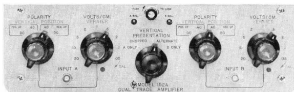
Fig. 3. Preamplifiers have convenient drawer style construction. DC-10 mc dual-trace unit shown above.
