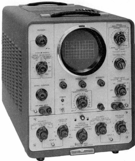
Fig. 1. (At left.) New -hp- Model 150A DC-10 Mc Oscilloscope has been designed with such special features as a 100x magnifier, automatic triggering, electronically re-armable single sweep, and plug-in preamplifiers. Many mechanical features are also included.
